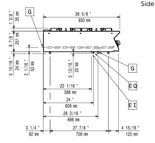
Electrical inlet (power) Gas connection
